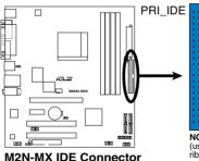
NOTE: Orient the red markings (usually zigzag) on the ID ribbon cable to PIN 1.
