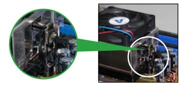
3. Align the other end of the retention bracket (near the retention bracket lock) to the retention module base. A clicking sound denotes that the retention bracket is in place.
