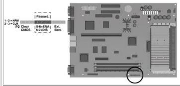
To set a new password, move the password header back to pins 5 and 6, restart the computer, and reestablish your password through Security Management.
