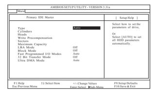
**[USER]:** It allows user to manually enter the number of cylinders, heads, and sectors per track for the drive.
