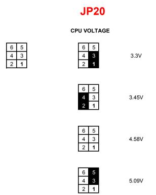
NOTE: cpu voltage measured with a multimeter on the pins S-10 (Vss) and R-10 (Vcc) of the Socket 3
