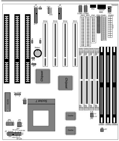
Figure 2–1. Mainboard Component Locations
