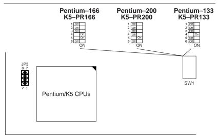
Figure 2–6. CPU Type Configuration
