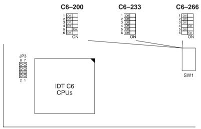
Figure 2–5. CPU Type Configuration
