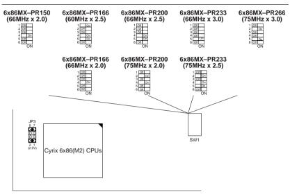
Figure 2–3. CPU Type Configuration
