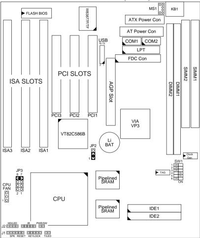
Figure 1–1. SL–54T5 Motherboard Layout
