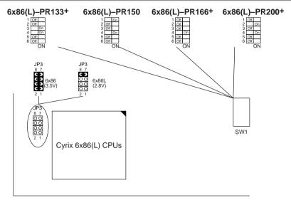
Figure 2–4. CPU Type Configuration
