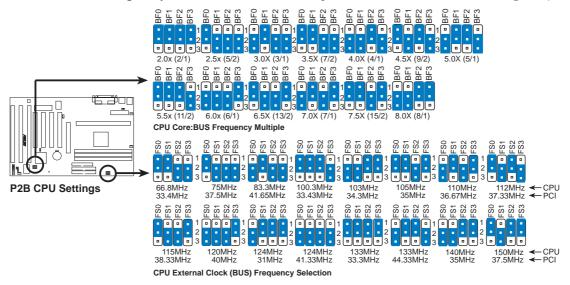
Set the jumpers by the Internal speed of your processor as follows:
